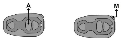
After the above two steps, the two headsets will automatically pair with each other until the LED on both headsets flashes blue At this point, two headsets can intercom with each other directly and both headsets can hear a voice notification <headset A pairing completed>.
